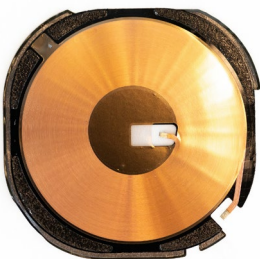
Wireless Charging Coil Gold Copper
